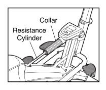
tance level is selected. CAUTION: The resistance cylinder becomes very hot during use. Allow the resistance cylinder to cool before touching it. When adjusting the resistance, touch only the resistance adjustment collar.
